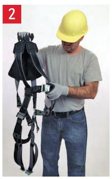
If chest, leg, and/or waist straps are buckled, release straps and unbuckle at this time.
