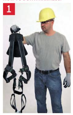
Hold harness by back D-ring. Shake harness to allow all straps to fall in place.
