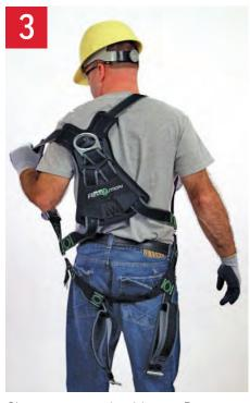
Slip straps over shoulders so D-ring is located in middle of back between shoulder blades.
