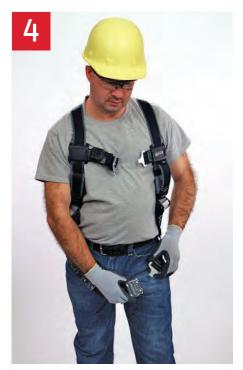
Pull leg strap between legs and connect to opposite end. Repeat with second leg strap. If belted harness, connect waist strap after leg straps.
