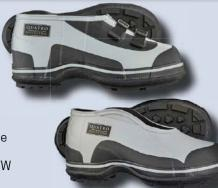
Dielectric overshoes slip on over work shoes protecting from risk of electrical shock when working on electric vehicles. Their insulating properties stop electrical current from being grounded. Various styles are available and meet ASTM F1116 standards.
