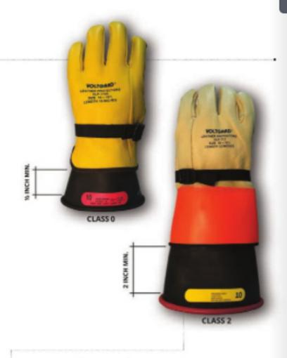
Minimum distances between the edge of leather protectors and the cuff edge of the rubber insulating gloves, according to ASTM specifications.
