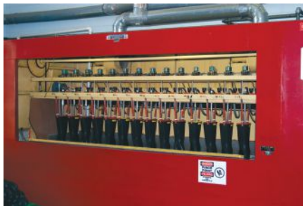
Glove electrical testing.
