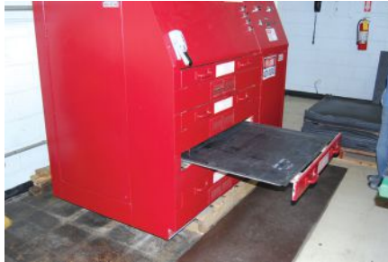
Blanket electrical testing.
