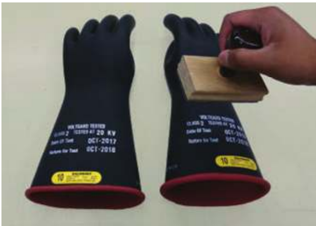
Goods should be marked according to your company's safety protocols, and previous testing markings should be removed prior to use.
