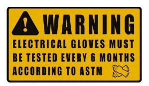
Rubber insulating gloves are the only protective gloves designed for constant contact with, and protection from, energized conductors and equipment. All of the other items are designed for protection from accidental, incidental or brush contact. Arc-rated work gloves alone offer no shock
