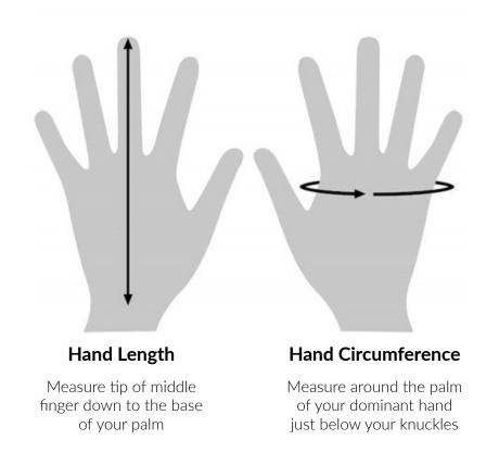
The ASTM D120 standard specification provides the measurements of the diameter of the palm for manufacturers, measured at the midpoint of the palm, plus or minus ½-inch. Measure the hand by wrapping the tape all the way around the palm. This number would equate to the probable size of the glove to select. Personal preference for tightness and finger length will ultimately determine the size that the wearer will choose.
