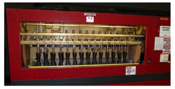
ASTM Manufacturing and Acceptance standards mandate the testing of the rubber insulating gloves by the manufacturer or supplier prior to the first delivery to the end user. Users also have the option of performing or requiring an acceptance test within
