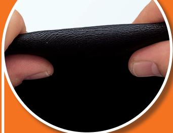
**— UV Checking:** Storing in areas exposed to prolonged sunlight causes UV checking.
