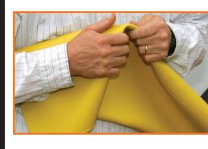
**Sleeve Inspection:** Inspect sleeves along the edge as they are rolled. Rolling will stretch the sleeve along the edge, making cuts, tears and
